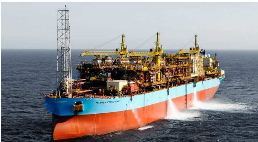
Maersk Peregrino has a production capacity of up to 100,000 barrels of oil per day.
